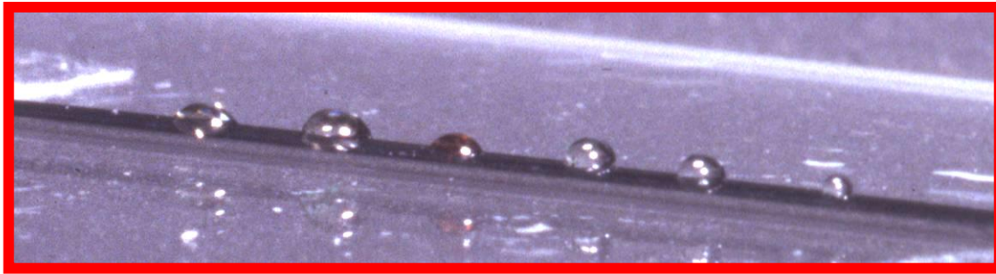
Close-up of a series of liquid droplets on a carbon-based coated sample
